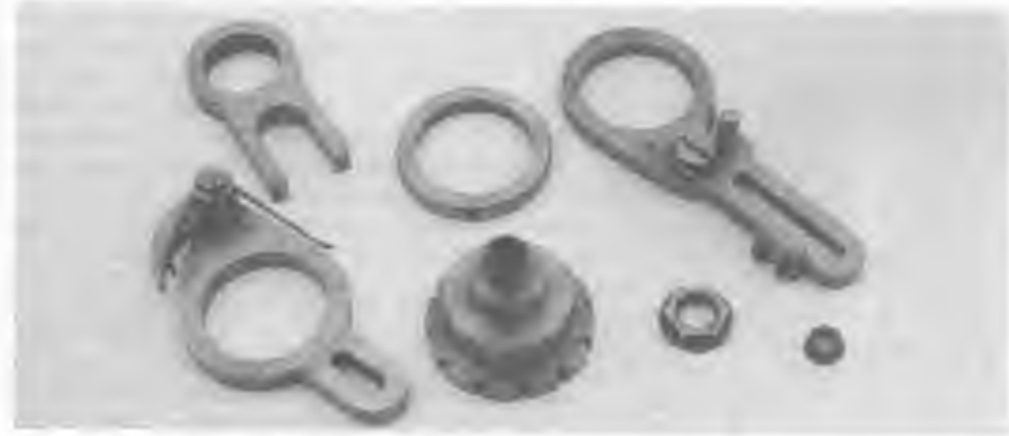
Fig. 107 Above, the spread of parts needed to make the Eureka form-relieving tool. Right, the completed machine with a cutter mounted, below in use on the lathe.
